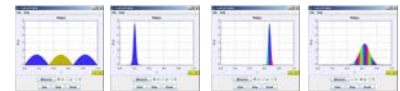
Figure 9: For the n = 3 energy eigenstate, the result of subsequently measuring x , then measuring p , and finally measuring x again, all on the same system.
