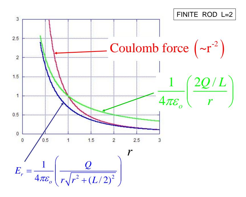
Electric field of a finite rod
